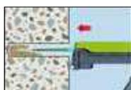
4. VMH in Bohrloch injizieren
